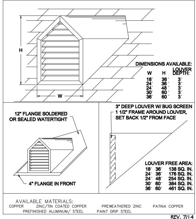
INSTALLATION: MARK OPENING IN ROOF DECK ON DESIRED COURSE. CUT OPENING IN
